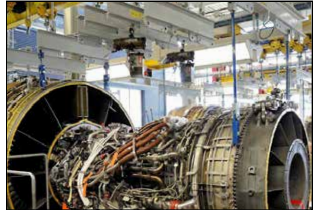
Monitoring loads while lifting - jet engine with four pick points
